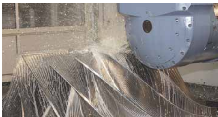
Inside the 5-axis machine: the milling process
