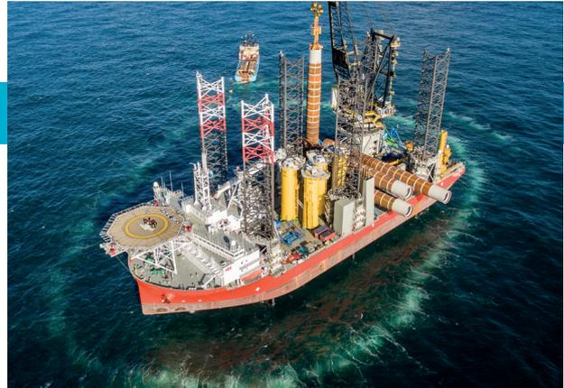
**Oil-free compressed air for bubble curtains in the North Sea. Bubble curtains protect marine life against noise and vibrations during the build-up of wind turbines. 13 compressors type PTS 1600 delivered 100% oil-free air for this specific project.**
