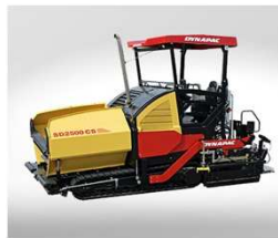
Dynapac asphalt paver
