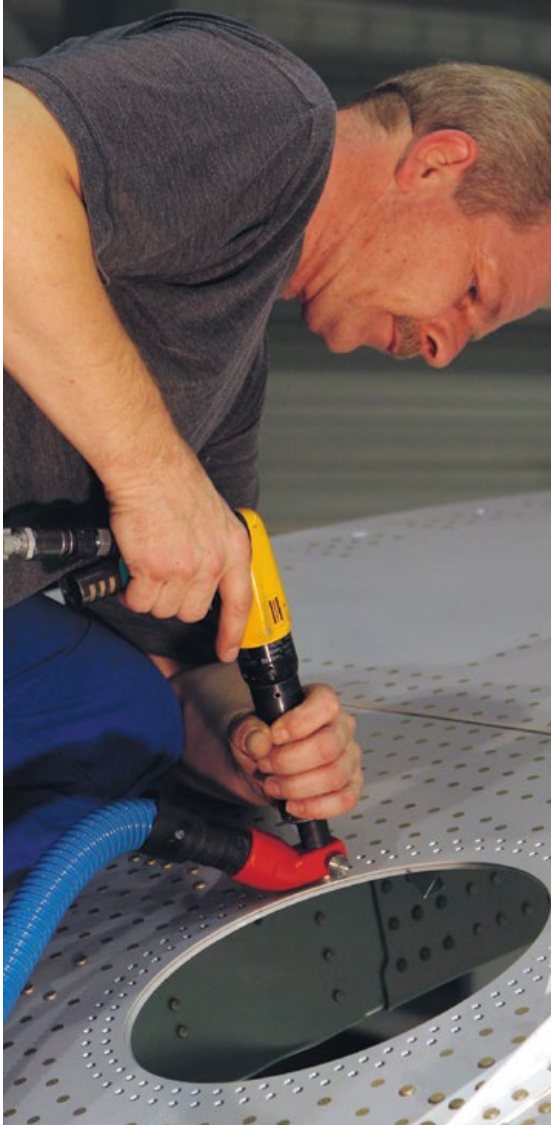
Working with high feed forces requires the operator to lean forward slightly in order to make use of his body weight.
