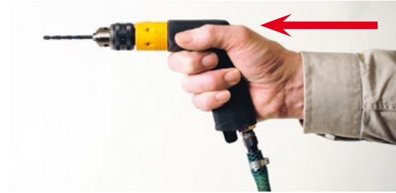
Fig. 3.3 The same feed force applied by the operator causes a different load on the wrist depending on posture.
