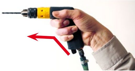
Fig. 3.3 The same feed force applied by the operator causes a different load on the wrist depending on posture.
