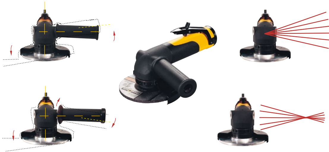
Fig. 3.17 Analysis of the grinder in running mode as seen from the front end. Above left: the machine is fitted with a stiff handle moving in phase. Below left: the machine is fitted with an anti-vibration handle moving out of phase. The question is, which solution is the best?
