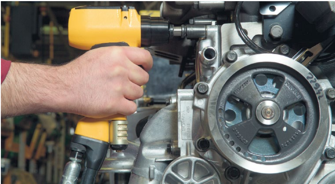
An oil cushion eliminates high-frequency noise from the process.
