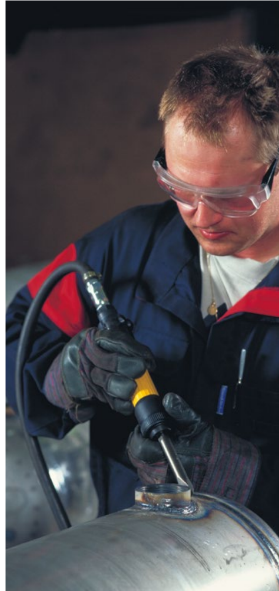
Scalers are commonly used in welding operations.
