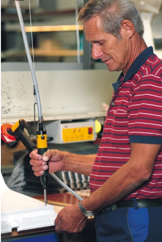
A modern screwdriver has a handle with a viscoelastic grip and a pronounced stop to reduce the grip force.
