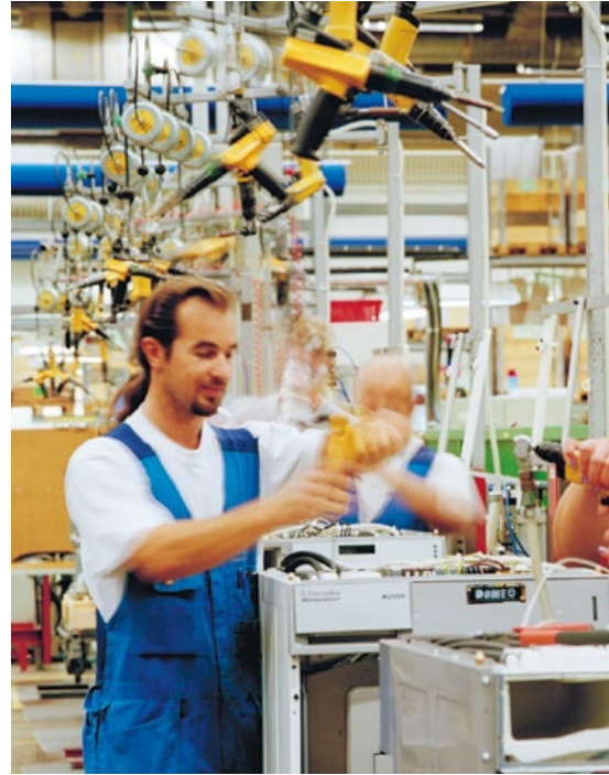
A balancer compensates for the weight of the tool.
