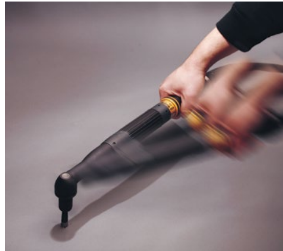
Rapid motions of the hand-arm system are perceived as shocks.
