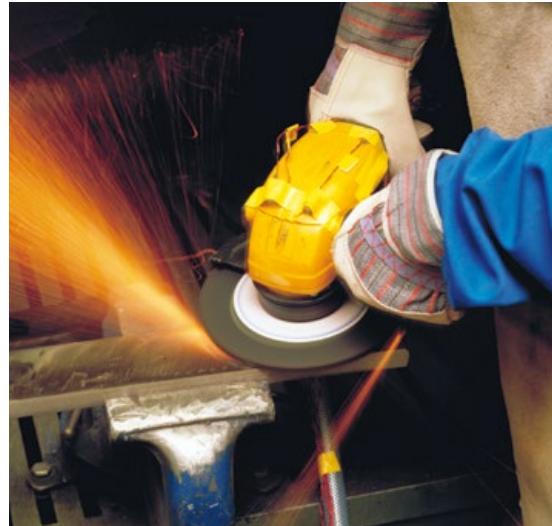
Grinding wheel imbalance is one of the main sources of vibration.
