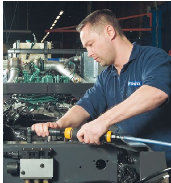
Angle nutrunners are widely used on assembly lines today.
