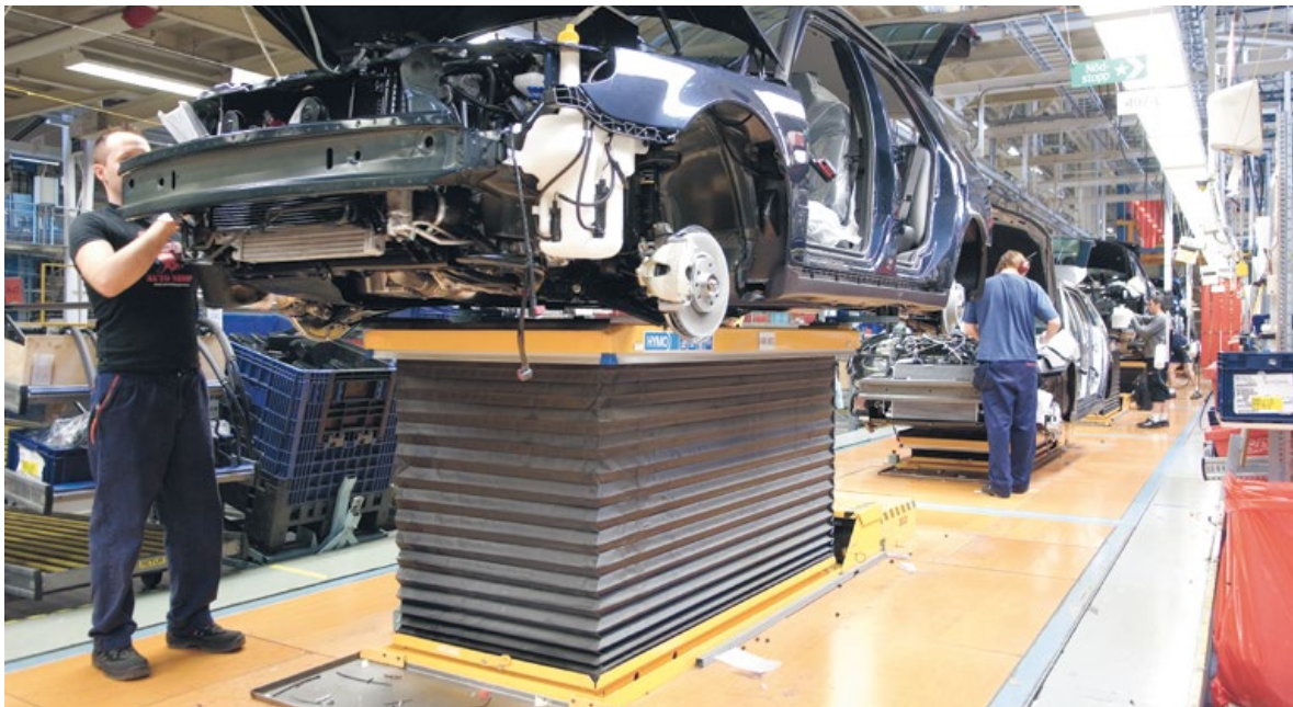
On modern production lines cars can often be adjusted in height to allow good postures for the assembly operators. This is especially important where high feed forces are applied.
