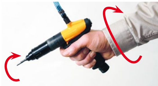
Fig. 3.4 When using pistol grip tools, torque applied by the operator is limited by the operator's supination torque capacity. For higher torque an angle nutrunner is a better alternative utilizing the pulling back force to balance the installed torque.
