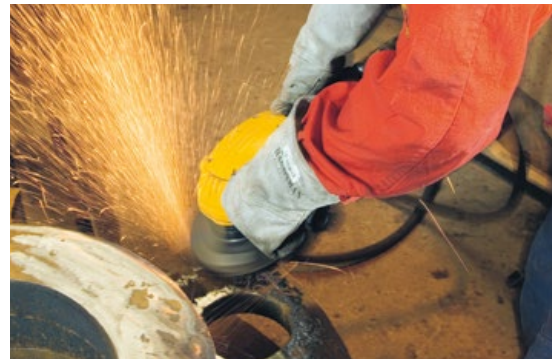
Modern turbine grinders can preferably be run on non-lubricated air.
