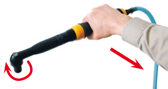
Fig. 3.4 When using pistol grip tools, torque applied by the operator is limited by the operator's supination torque capacity. For higher torque an angle nutrunner is a better alternative utilizing the pulling back force to balance the installed torque.
