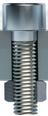
More than 80-90% of the tightening torque goes to overcoming the coefficient of friction underhead and thread.
