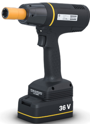
The Tensor TBP cordless pulse tool is a battery powered, low reaction tool with high torque capacity. The accuracy has been verified to be within 7.5% for the TBP6, TBP8 and TBP9.
