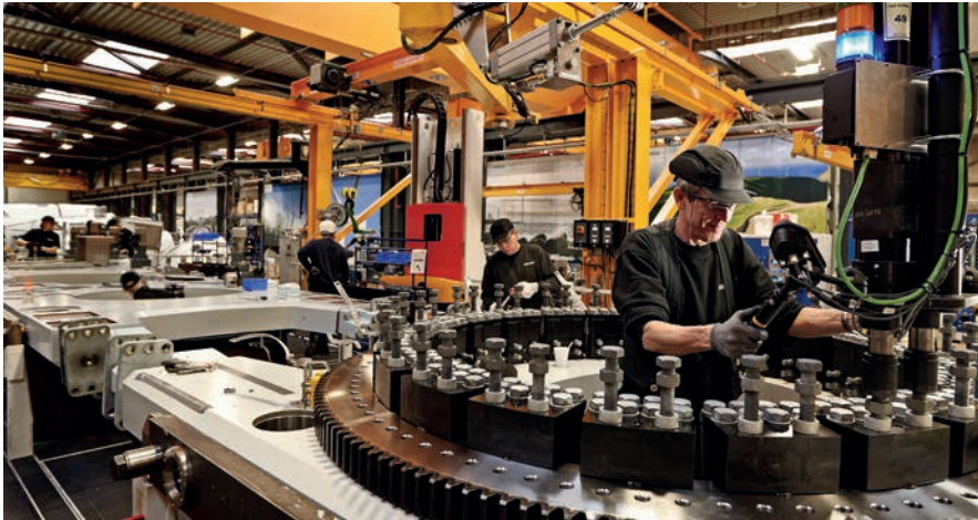
Major OEMs use smart tooling in their assembly lines today, with full error proofing and data capture
