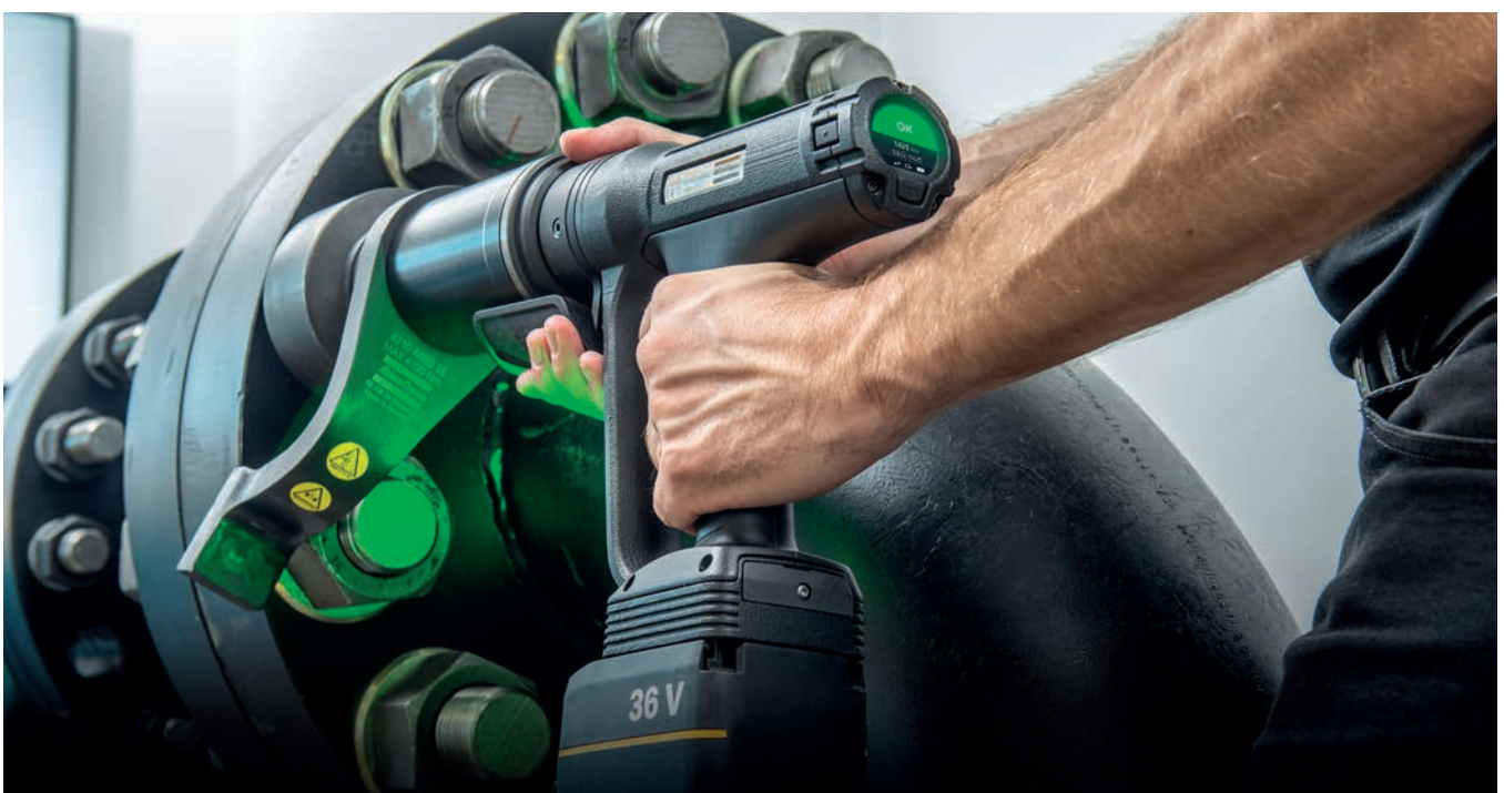
Our recently launched smart high torque battery tool can significantly reduce process times for service operations
