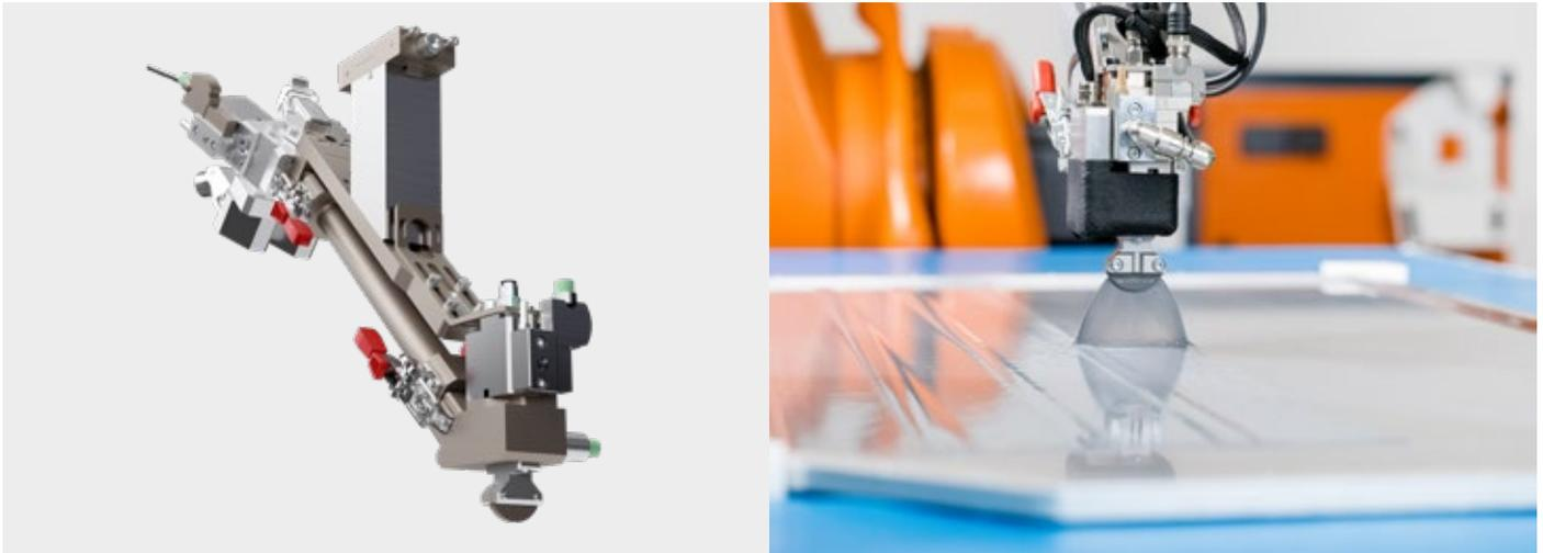
The SCA FlexS.Seal is an applicator especially developed for the wide flat stream application of liquid 2K fire protection materials in battery assembly.
