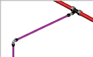
DETAIL VIEW - REDUCTION TEE to 50 mm AIRnet / DROP LEGS (TYP)
