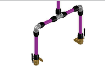
DETAIL VIEW - 50 mm DROP TERMINATIONS / 2 F-NPT VALVES
